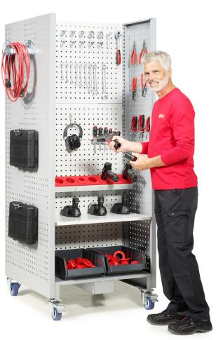
The frame is made of powder-coated steel (grey, RAL7045). Accessories and add-on products are available in light grey (RAL7035, Treston colour code -49). Because the frame is equipped with the M750 upright frame module, almost all modular size M750 accessories are compatible with the Treston Tower storage and workstation unit.
